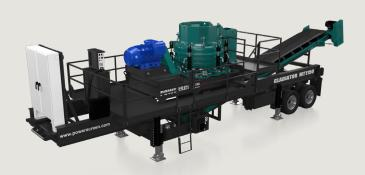
The Gladiator MT1150 is a new electrically driven, wheeled open circuit cone crusher. It features the renowned Terex (r) TC1150 cone chamber and is chassis mounted on wheels meaning ease of movement and quick set up times.
