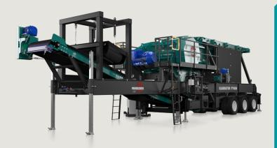
The Gladiator PT450 is a new electrically driven, portable jaw crusher. It features the tried-and-tested Terex CR040 jaw crushing chamber and is chassis mounted on wheels meaning ease of movement and set-up.
