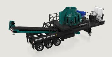
The new Gladiator MT1300 is an electrically driven, wheeled open circuit cone crusher. It features the tried and tested Terex TC1300 cone chamber and is mounted on wheels which ensures ease of movement and quick set up times.
